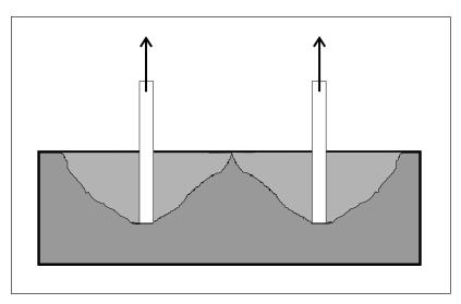
When anchors are close to one another, or to edges, the cone of the concrete cannot form fully. Therefore a reduction in the ultimate load bearing capacity of the anchor is anticipated.
