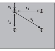
Anchor #4 is the most effected by edge and spacing conditions in the anchor group.
