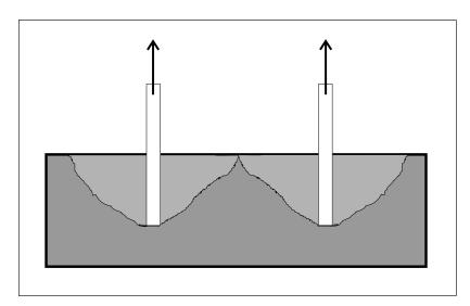
When anchors are close to one another, or to edges, the cone of the concrete cannot form fully. Therefore a reduction in the ultimate load bearing capacity of the anchor is anticipated.
