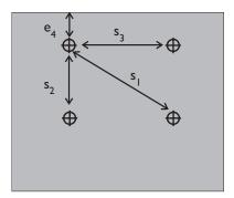
Anchor #4 is the most effected by edge and spacing conditions in the anchor group.
