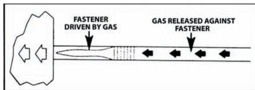
2. Indirect acting tools have a captive piston which is driven by the expanding cartridge gas. The piston then drives the fastener into the work surface.
