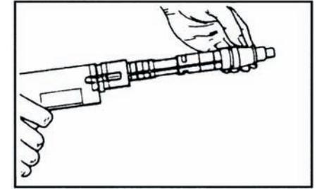
1. With the point out, insert fastener into the guide until it is held in place by the plastic washer.
